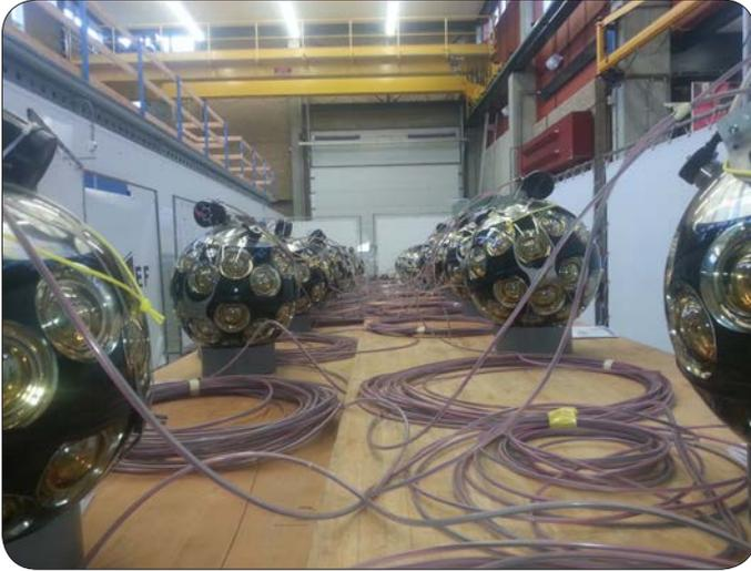
*Figure 2. The first fully assembled KM3NeT string with 18 optical modules at Nikhef.*
