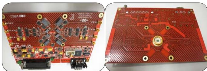
Figure 4. Front- and back-side of the PCB for the linear-alignment front-end systems. The right panel shows the quadrant photo-diode.
