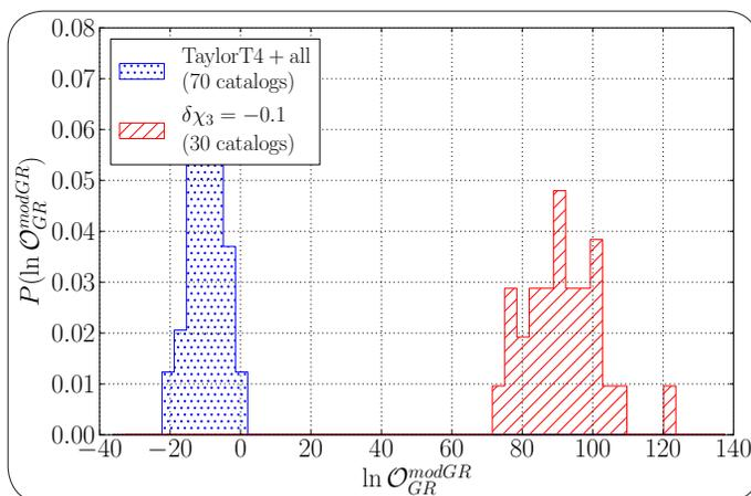
Figure 5. If the strong-field dynamics of spacetime is not as predicted by general relativity (GR), then the TIGER data analysis pipeline will be able to find out by studying gravitational wave signals from coalescing binary neutron stars. Shown are the distributions of TIGER's 'detection statistic' for GR violations, for the case where GR is correct (blue), and assuming a violation of the GR prediction for the self-interaction of spacetime (red).
