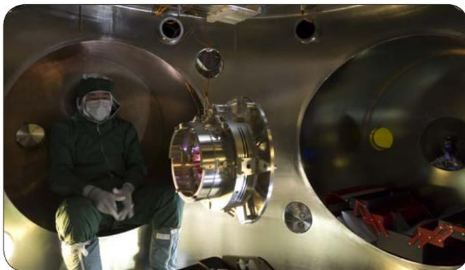
Figure 1. Installation of the new end-mirror suspension in Virgo's Input Mode Cleaner.
